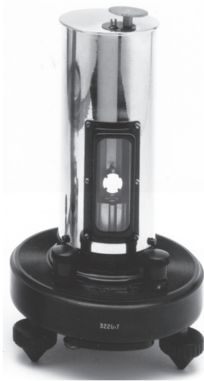
Figure B1. The Light Beam Galvanometer is Essentially a Sensitive Meter Movement. It Takes Gain in the Optical Angle of a Mirror Reflected, Collimated Light Source (Courtesy the J. M. Williams Collection)
