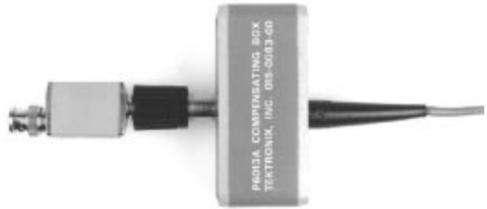
Figure C4. The Impedance Matching Box (Extreme Left) Mated to the High Voltage Probe. Note Direct Connection. No Cable is used
