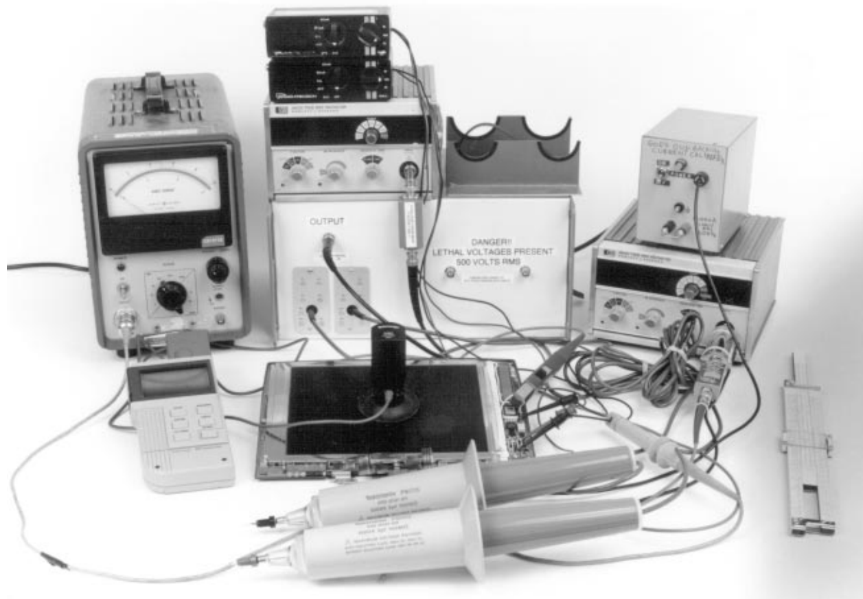
Figure D7. Complete CCFL Test Set Includes Photometer (Left and Center), Differential Voltage Probe/Amplifier (Upper and Lower Center), Current Probe Electronics (Right) and Input V and I DC Instrumentation (Upper Left). Computer (Lower Right) Permits Calculation of Electrical and Optical Efficiency
