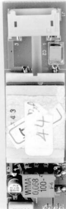
Figure G5. Transformer Output Terminals, Ballast Capacitor and Connector Are Isolated at End of Board. Slit Prevents Leakage
