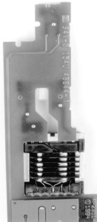
Figure G12. Bottom of G11 Shows Routed Area. Traces at Board Extreme Left Are Undesirable but Acceptable. Isolation Slit Between Traces and HV Points Would Be Preferable
