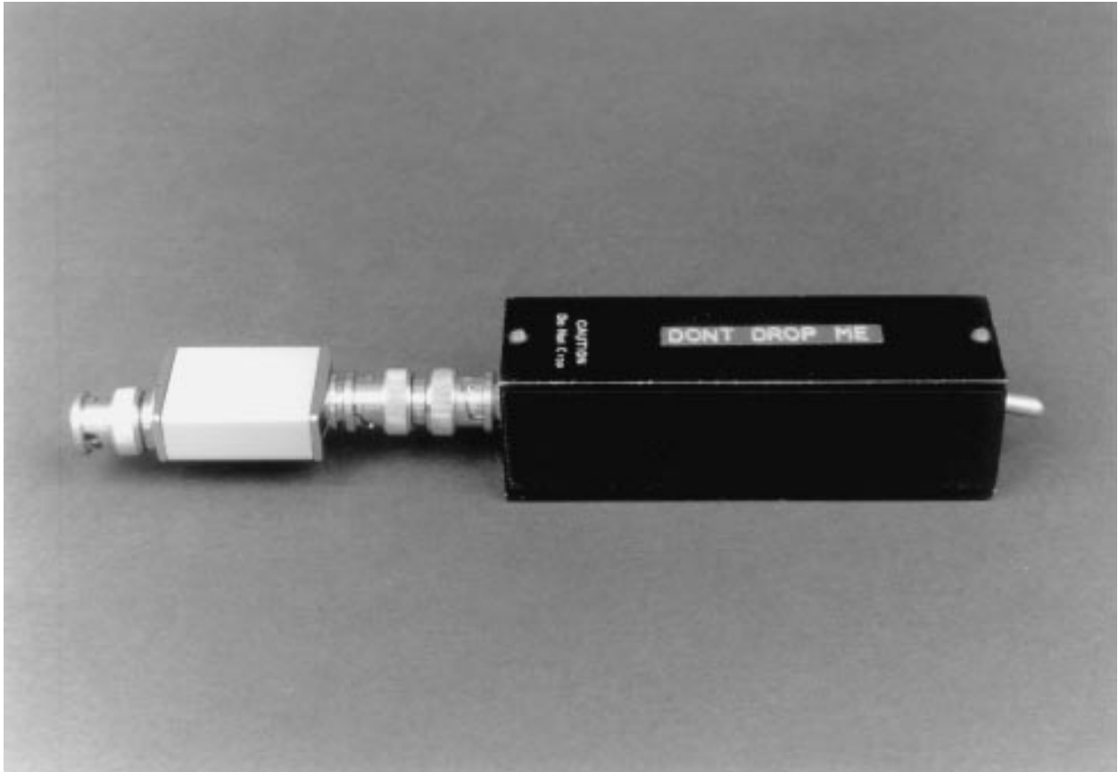
Figure B4. The Packaged Avalanche Pulser. 1.5V-to-90V Converter Is in the Black Box. Avalanche Head Is at Left
