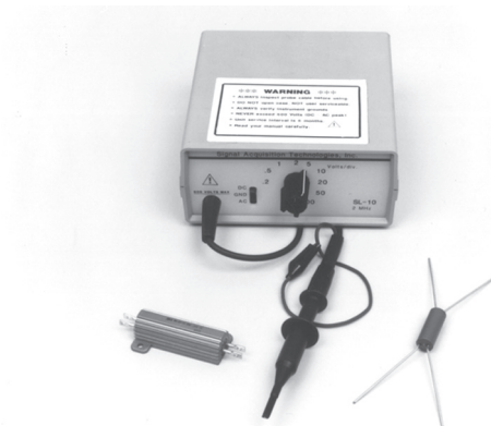
Figure C3. Typical Current Shunts and an "Isolated" Probe
