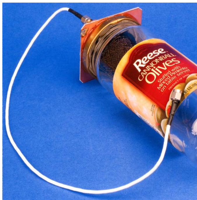
Figure 2. Photograph Details Cap Assembly, Partially Views Glass Enclosed Measurement Path. Ultrasonic Transducer Visible Within Cap. Stiffening Plate, Bonded to Cap Top, Prevents Ambient Pressure or Temperature Changes from Deforming Thin Metal Cap, Promoting Measurement Path Length Stability. Coaxial Header Provides Transducer Connections
