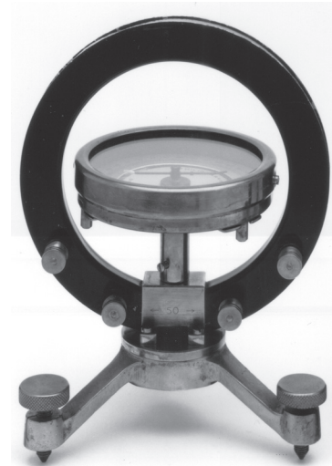
Figure B2. A Tangent Galvanometer Measures Small Currents by Indicating the Interaction Between Applied Current and the Earth's Magnetic Field. Absolute Current Value is Proportional to the Tangent of the Compass Deflection Angle (Courtesy the J. M. Williams Collection)
