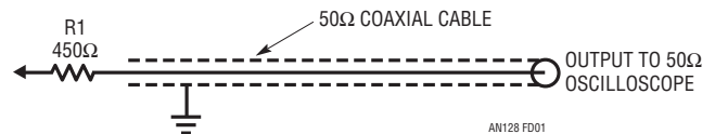
Figure D1. Conceptual 500\Omega , “ Z_0 ”, 10x Oscilloscope Probe. If R1 = 4950\Omega , 5k Input Resistance with 100x Signal Attenuation Results. Terminated Into 50\Omega , Probe Theoretically Constitutes Distortionless Transmission Line. “Do-It-Yourself” Probes Suffer Uncompensated Parasitics, Causing Unfaithful Response Above \approx 100MHz ( t_{RISE} = 3.5ns )
